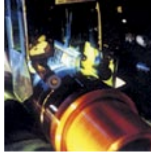
▲ Magnetic particle inspection (MPI)
